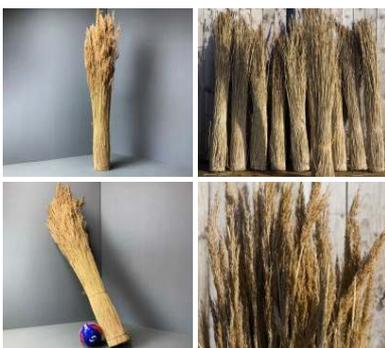
**Water Reed Bundle, approx. 2 m plus tall by 25 cm diameter. Complete with seed head. Natural, dried, thatching material**
